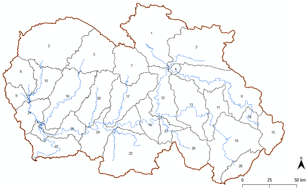
Figure 4: Overview of the sub-catchments in the SWAT model of the study area
