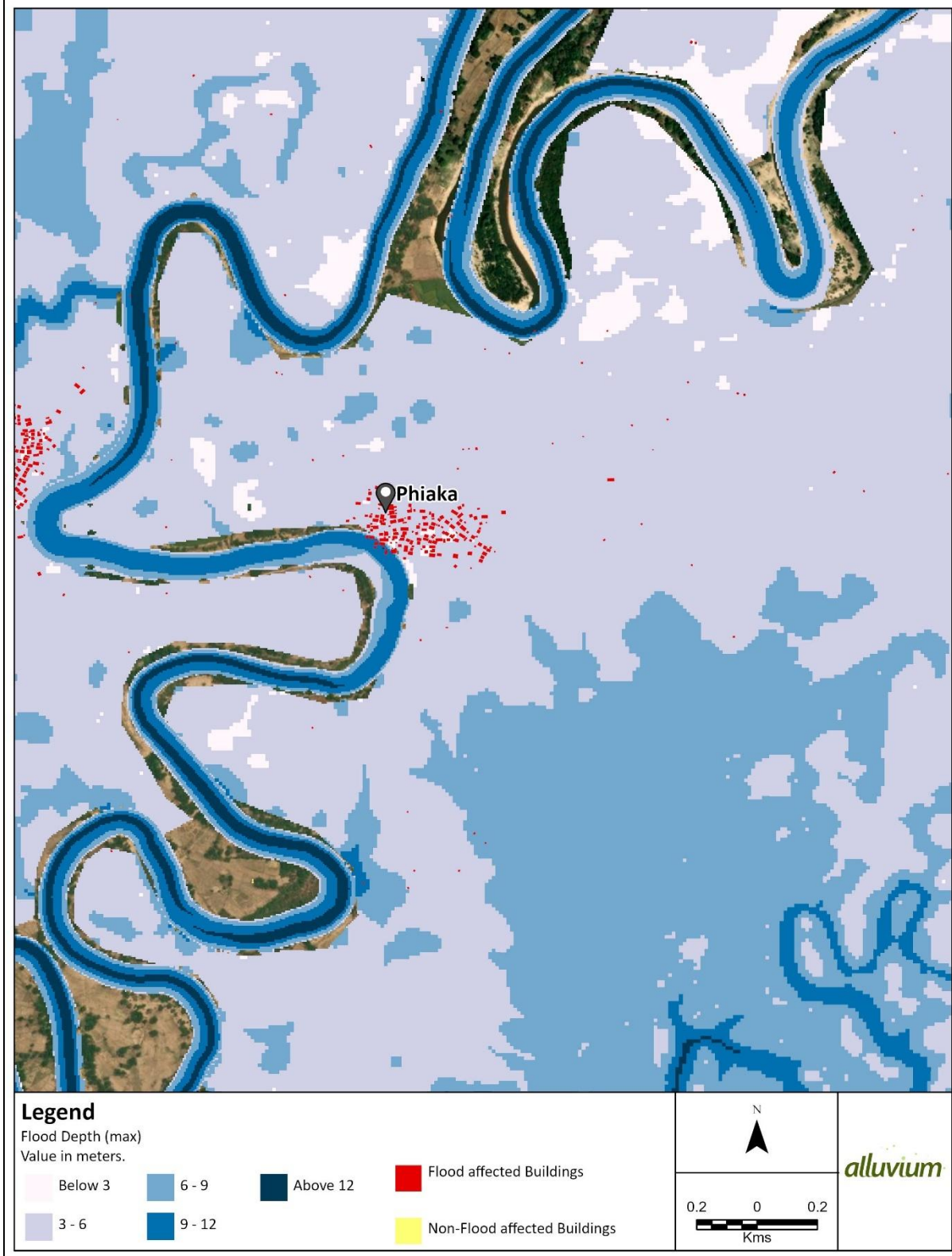
Figure 16. Flood extent and depth for storm event with a 100-year return period (current climate) for Phiaka Viillage
