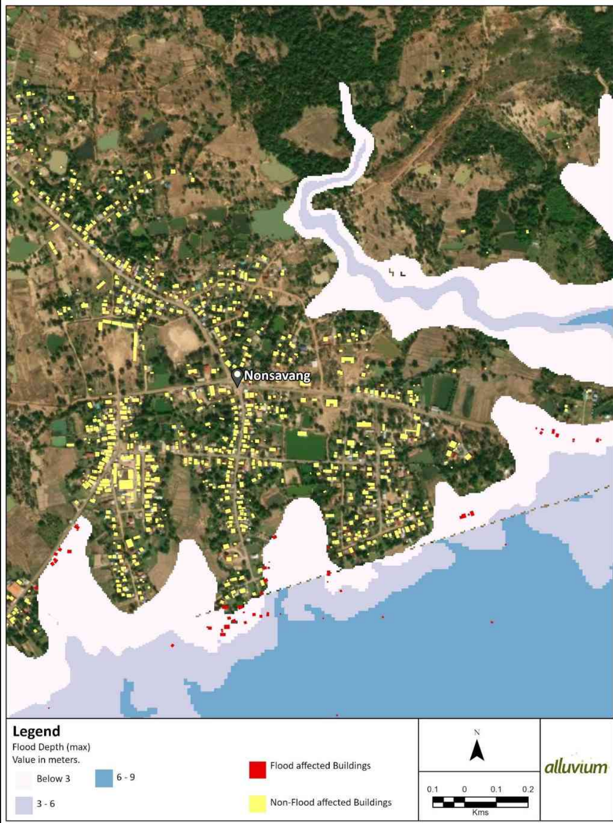
Figure 16. Flood extent and depth for storm event with a 100-year return period (current climate) for Nonsavang Village
