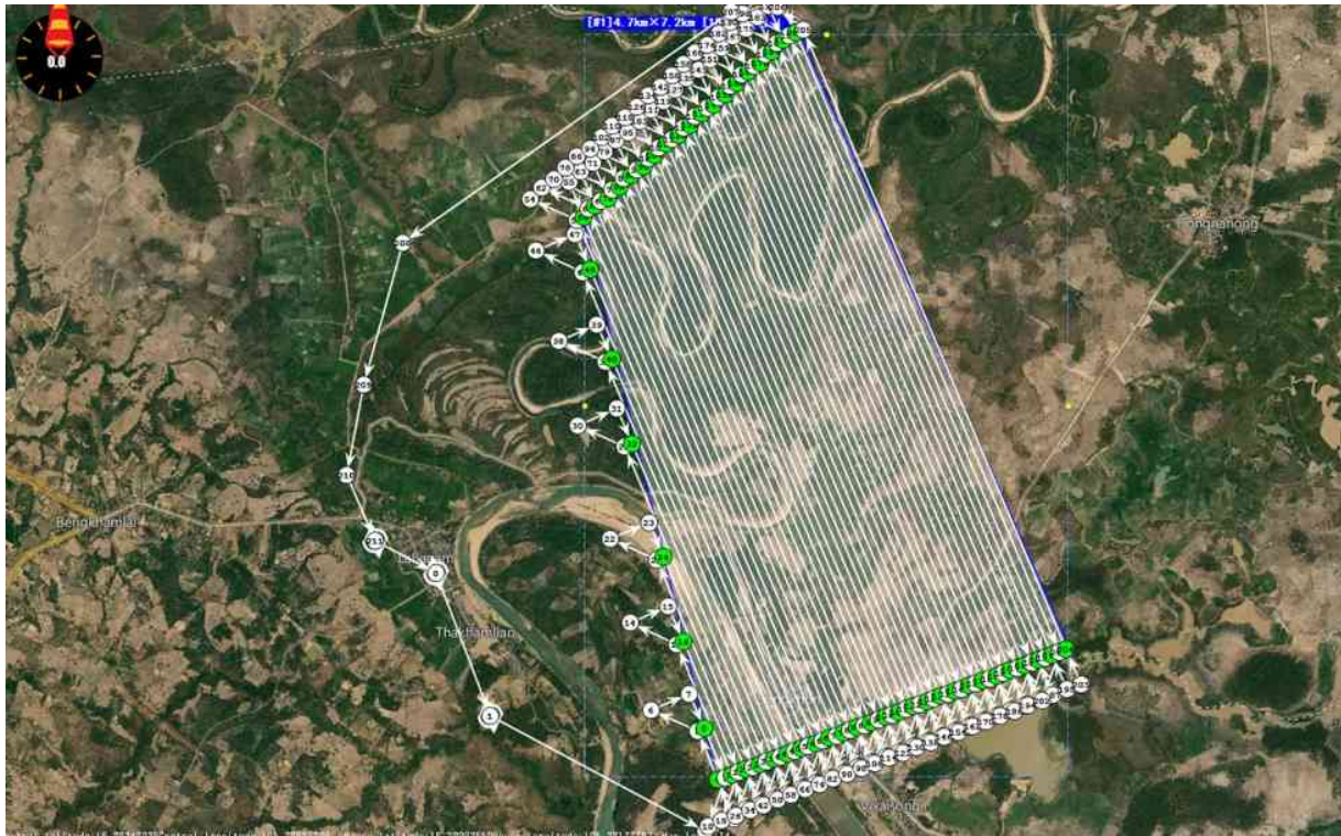
Figure 4: Flying plan one of the site areas as in SongKhone Village, SongKhone District (For detail Flight plan Show in Annex of each site area)
