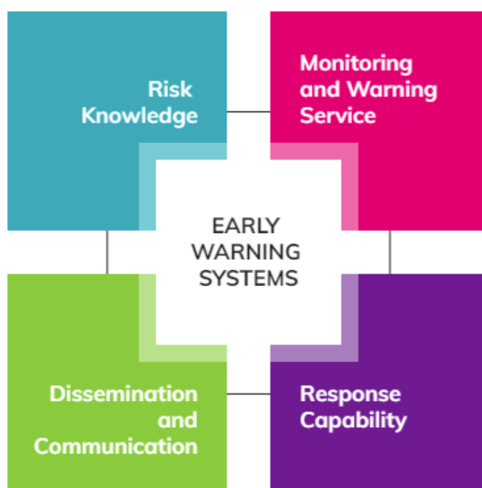
Figure 1. UNDP framework for early warning systems 1
